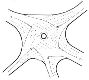
Saturation flow = total flow when there are queues at every branch ("Cardiff Roundabout" experiment, May-June 1969, Road Research Laboratory)
