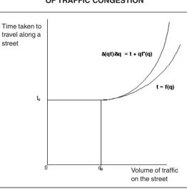
Figure II.1 SCHEMATIC REPRESENTATION OF THE CONCEPT OF TRAFFIC CONGESTION
