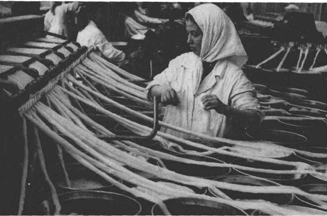
Drawing and blending of card slivers in a textile plant in Turkey
