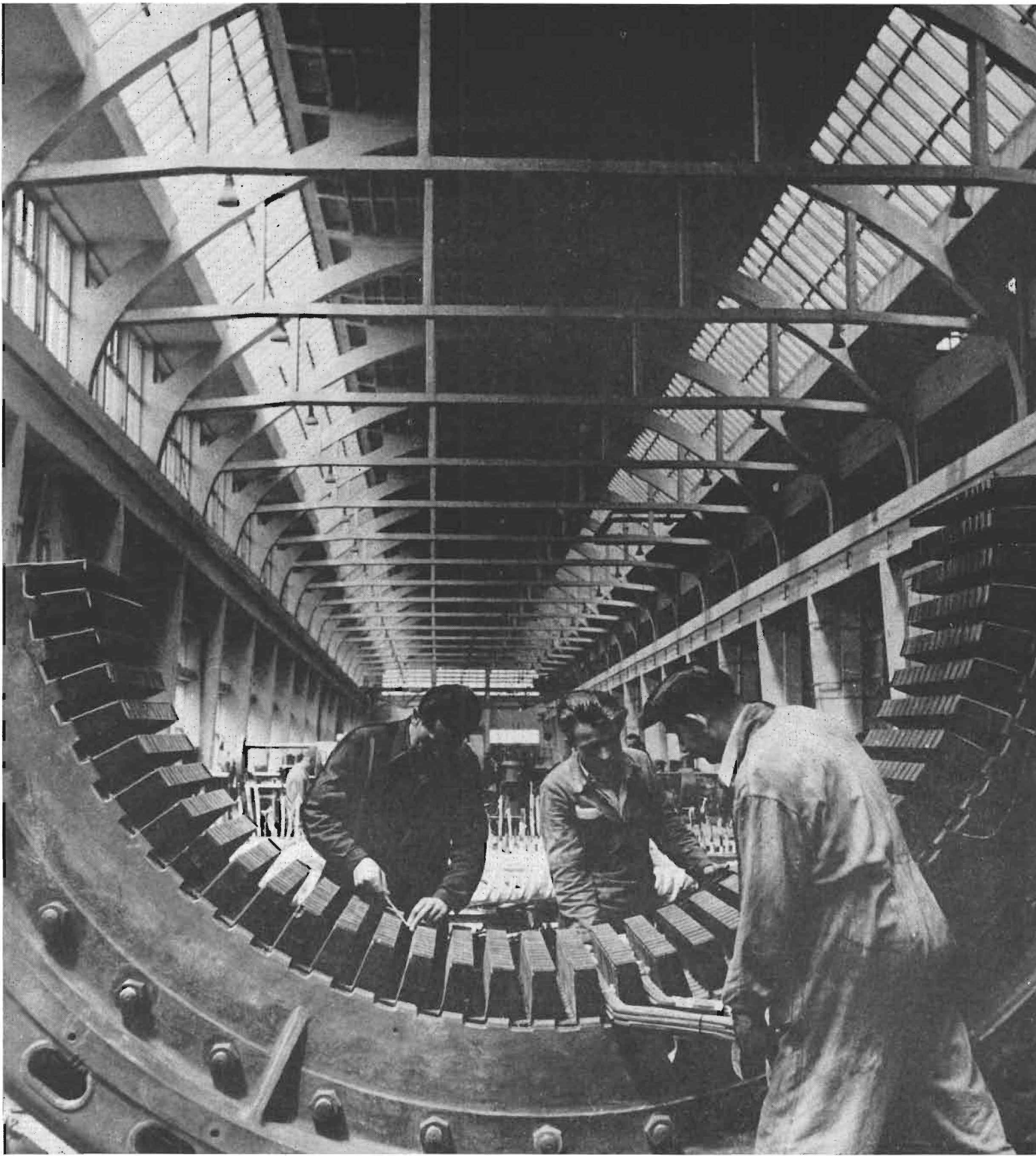
Placing field coils into an electrical generator in a Zagreb factory
