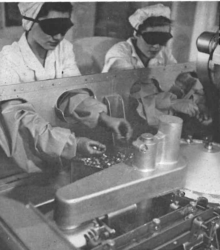
Capping penicillin bottles in a plant at Zemun: the workers wear rubber gloves to prevent contamination of the drug and dark glasses to shield their eyes from the ultra-violet light inside the cabinet
