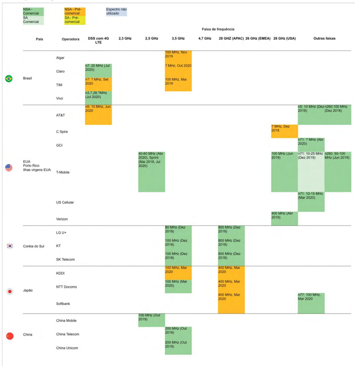
Fonte: List of 5G NR networks. Disponível em: <<https://bit.ly/3mm1cNB>>. Nota: <sup>1</sup> n5: 850 MHz FDD; n71: 600 MHz FDD; n77: 3,7 GHz TDD; n260: 39 GHz.
