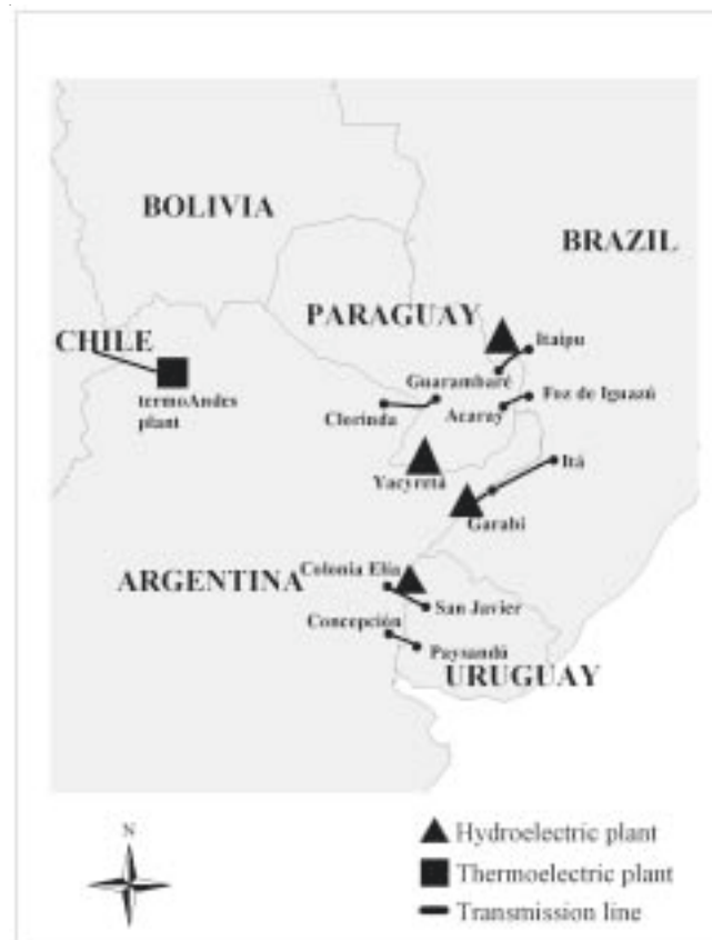
Figure III.3 SOUTHERN CONE: ELECTRICITY INTERCONNECTIONS
